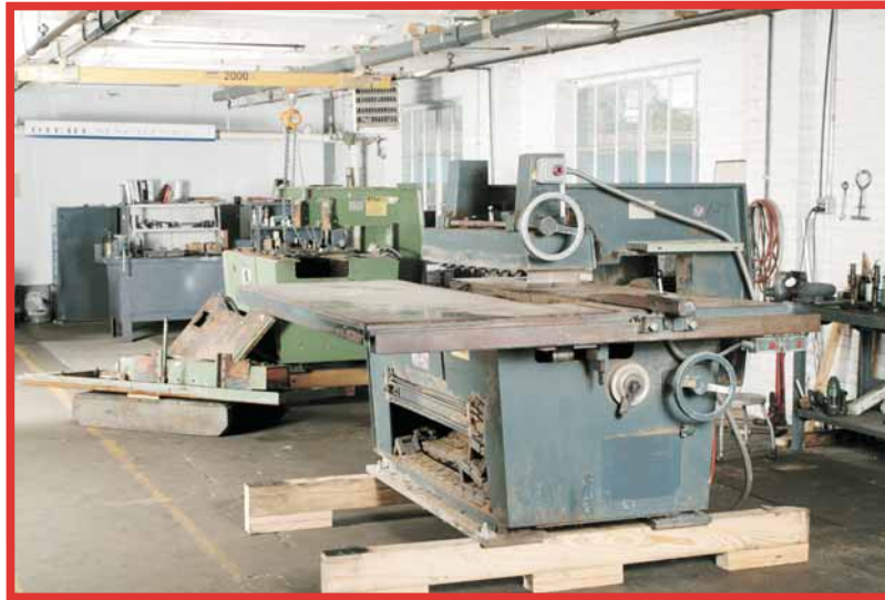
▲ A Diehl SL-52 Straight Line Rip Saw returned to the factory after years of hard production use. Positioned in-line and ready for remanufacturing.
