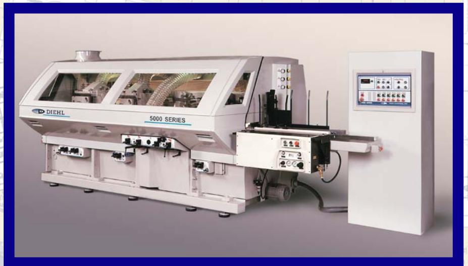
Front mounted controls are accessible with the enclosure in either the open or closed position. To further ease the set up function, the enclosure door opens and closes automatically with the push of a button.
