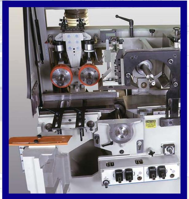
Better accessibility and larger cutterhead swings on the horizontal spindles offer the operator faster setups and greater profile flexibility.
