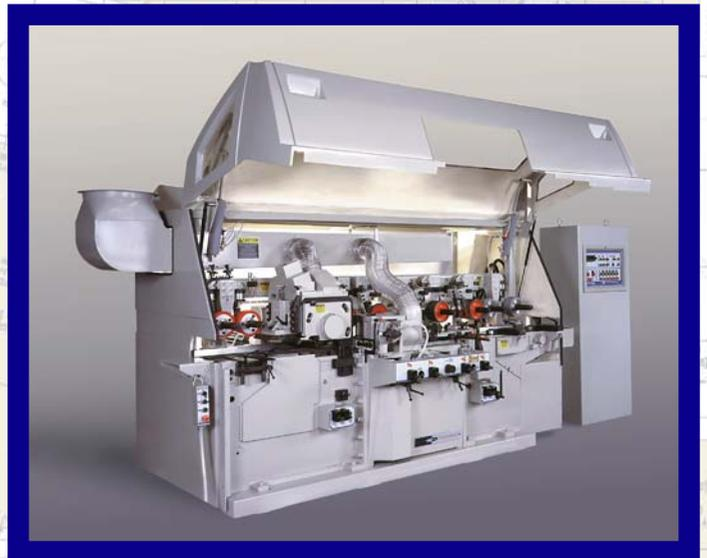
Each 5000 Series model is equipped with a complete enclosure for operator safety and noise abatement. An interior dust manifold, provided as a standard feature, reduces the length of each cutting head's dust connection, and requires only one external connection point. This reduces your installation costs, and greatly improves the dust collecting performance.
