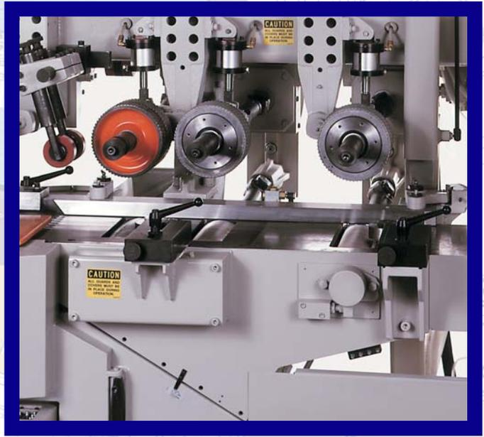
The 5000 moulder can be provided with optional dual or triple upper and full width lower feed rolls to provide smooth, positive feeding of the stock. Also available is an "air dried" lumber feed package, enabling individual height adjustment for the lower feed rolls.
