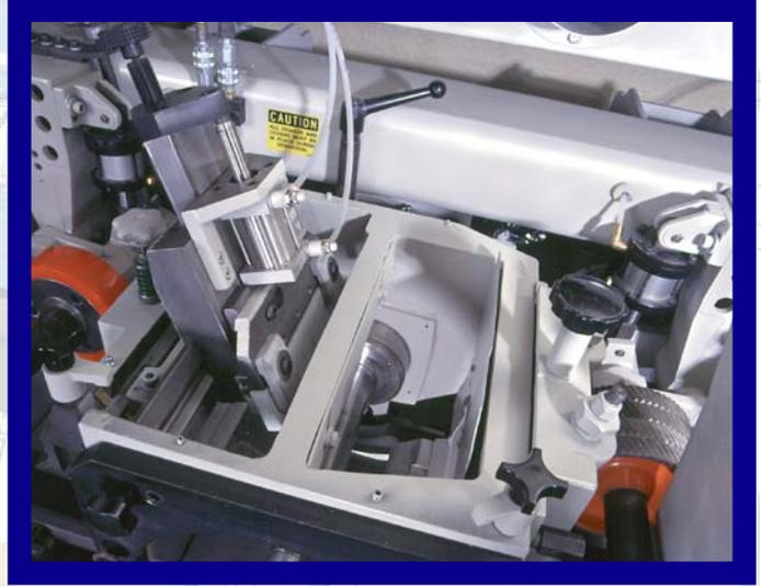
Automatic jointers are available for high-speed applications and have smooth, vibration-free movement of the stone into the knives. The stone depth advance is infinitely variable by the operator, giving complete control in achieving "hair line" jointing.
