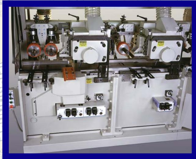
Horizontal spindle outboard bearings, with axial adjustment, are available for achieving the perfect finish when machining either at high speeds or in challenging profiles.
