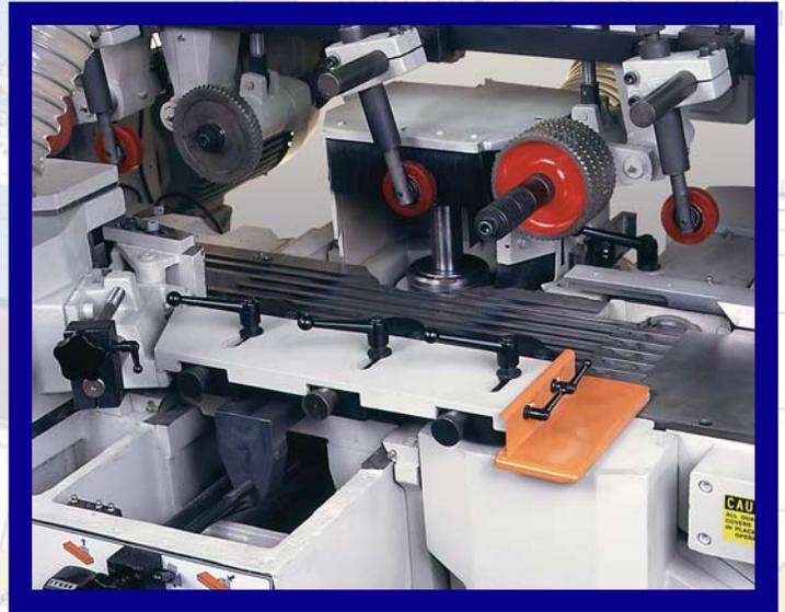
A grooved bed stock guide system is available for applications where short stock or twisted stock is being processed.
