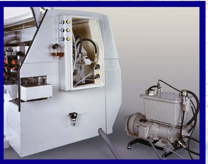
Hydraulic Drives are available for the more demanding applications and use 6 3/8" diameter feed rolls for feed speeds up to 350 fpm.
