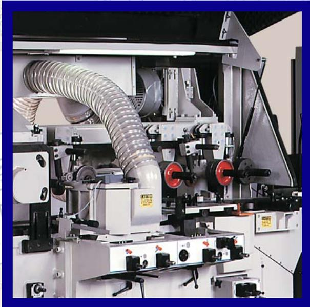
An A.C. frequency inverter drive that includes 5 1/2" diameter feed rolls, is standard for applications up to 225 fpm, assuring smooth vibration-free feed system.
