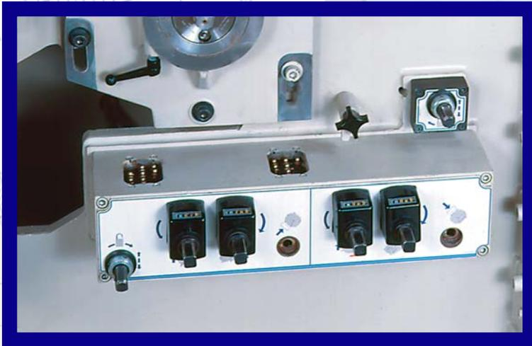
A centralized lubrication system, with grease fittings located convenient to the operator, assures easy access to all of the stationary grease points on the machine.
