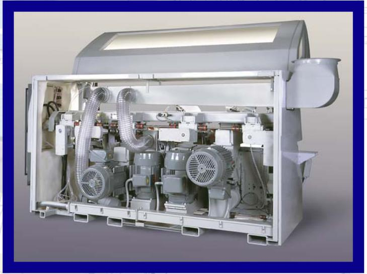
The heavy-duty design/construction allows for mounting large horsepower motors (up to 50 hp) used for high-speed production (up to 350 fpm), or deep-profile moulding.
