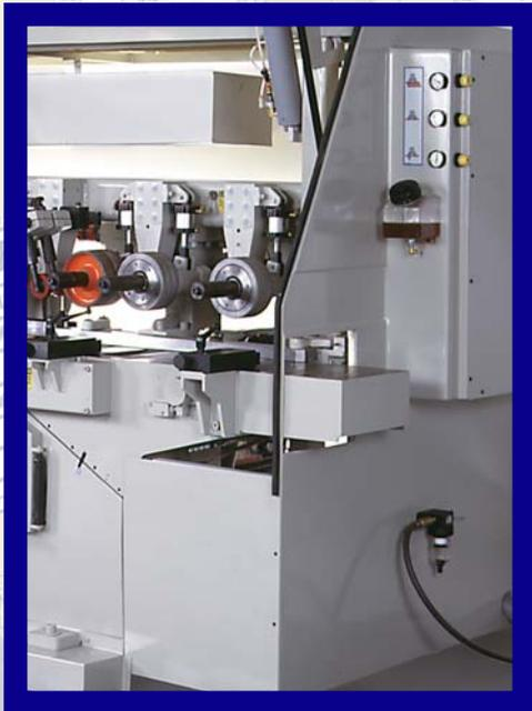
A shortened infeed table is available for high-speed operations using automated lateral chain-feed systems.
