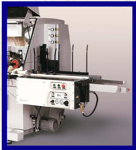
The infeed table can be extended for manual loading or for a magazine loading hopper.
