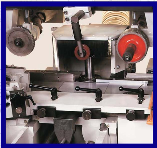
Spring or Pneumatic holdover and chipbreaker groups are available to securely hold the stock while machining.
