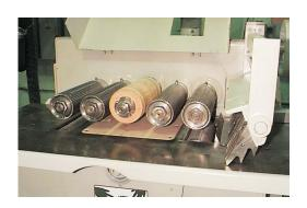
An additional center feed roll can be added for ripping short length stock. The center roll uses a removable sleeve to mount spur drive discs, wooden rolls (shown above) or urethane feed tires. This option accommodates ripping stock as short as 8" long.
