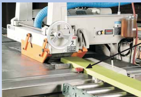
Close-up with side pressure roller engaged against material.
